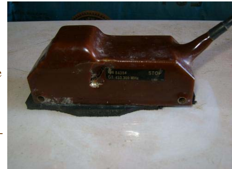
Figure 1: Damaged satellite transmitter showing bullet hole
